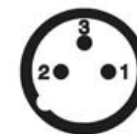
DMX - output XLR mounting-sockets (rear view):
