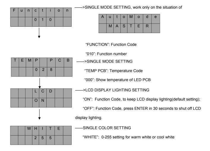
Press the "MODE" then press the "ENTER" to begin your setting. Press "UP" and "DOWN" to switch the modes with the shining Function Code. Be sure to press the "ENTER" button to save your changing, it won't be saved if the button has not been pressed. Moreover, the saving data still exists even after power off and then on.
